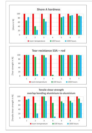
Medium 1: Engine oil at +105°C Medium 2: Engine oil at +150°C Medium 3: Water/glycol at +105°C Medium 4: Water/glycol at +150°C Medium 5: Cold degreasing agent at room temperature Medium 6: Brake fluid at room temperature Medium 7: Drilling coolant at room temperature
