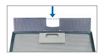
Mark the Filter size on the new expanded metal layer. Filter size = Frame size minus 3 mm for the longitudinally side and minus 5 mm for the opposite handle side.
