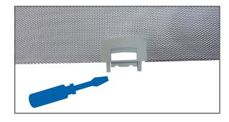
Spread the frame carefully (not more than the width of the handle), to avoid breaking the edges. Pull out the old filter mat carefully and place the handle aside.
