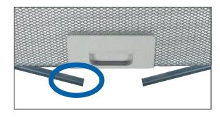
Place the cutted new filter mat carefully into the frame. Insert one of the included handle (for the appropriate frame 8mm or 9mm) into the cutted area. Close the frame carefully and screw the screws tight.
