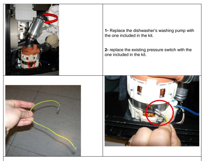
**3-** Connect one end of the ground cable provided to the pump ground connector and the other to the heating element ground connector
